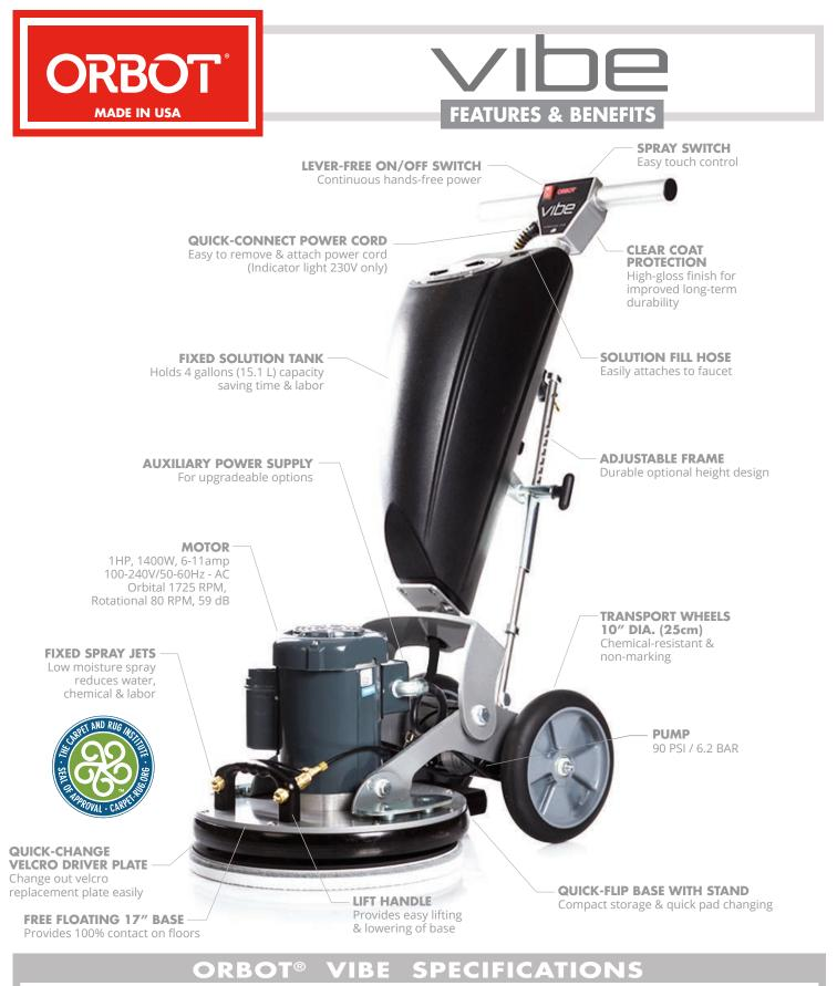
**DRIVER DIAMETER** 17 in / 43.18 cm • **MOTOR** 1HP, 1400W 100-240V / 50-60Hz, AC • **DUAL SPEED** Orbital 1725 RPM + Rotational 80 RPM **NOISE LEVEL** 59 dB • **WEIGHT** 95 lbs / 43.09 Kg • **WHEEL DIAMETER** 10 in / 25.4 cm • **SOLUTION TANK CAPACITY** 4 Gal / 15.1 L **PUMP** 90 PSI / 6.2 BAR • **QUICK-CONNECT POWER CORD** 50 ft / 15 m • **WARRANTY** 2 Year (see Warranty for Coverage)
